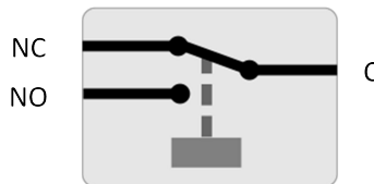
Internal operation of the programmable relay
